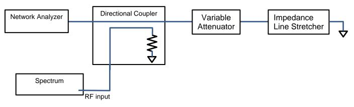
Fig.1. Variable Attenuator Adjustment Setup
