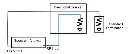
Fig.6. Spurious Level Measurement Setup
