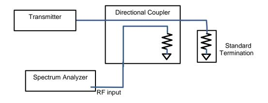
Fig.3. Reference Level Setting Connections
