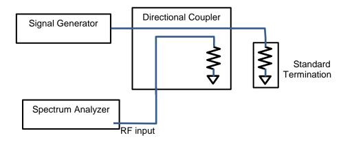
Fig.5. Spurious Level Measurement Setup
